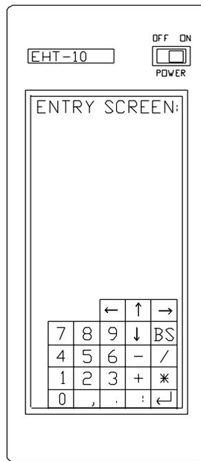
Figure 3 FST Numeric Entry Screen
