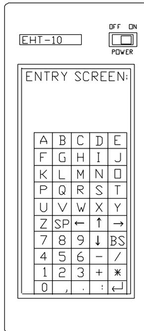
Figure 2 FST Alphanumeric Entry Screen
