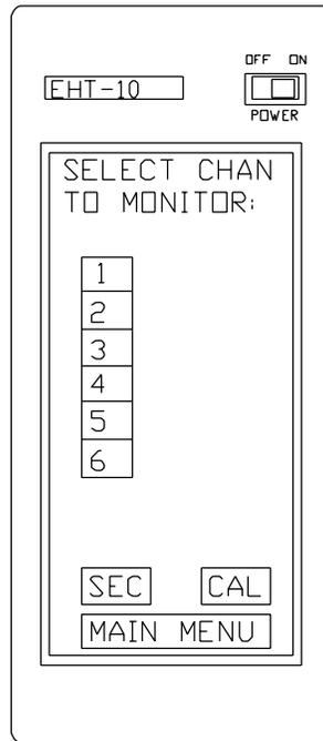
Figure 18 Select Channel To Monitor Screen
