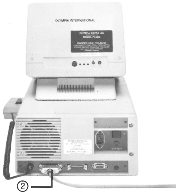
Plug 2 for parallel connection Centronics interface 7-bit ASCII, TTL
