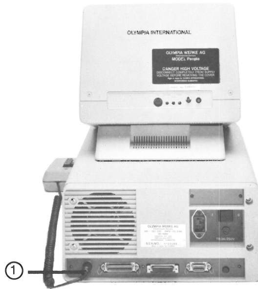
Plug 1 Connection of the keyboard to the main unit (back side)
