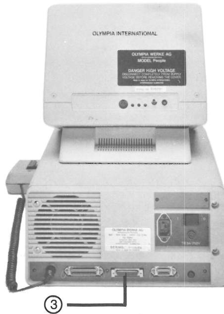
Plug 3 for RS-232-C interface, (V24) asynchronous-synchronous from 150 to 9600 Baud
