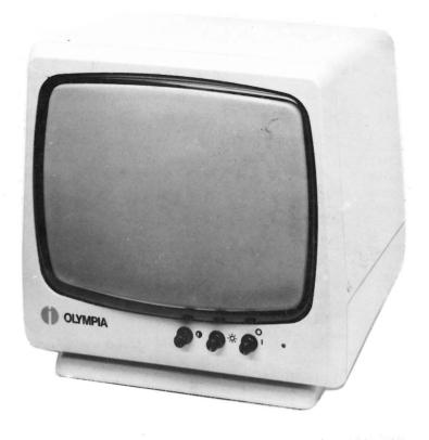
The CRT is to be placed with its base free to move in all directions, so that the user can adjust it to the most favorable position. The CRT is connected to the main unit via a plug-in type of connecting cable. The unit has its own ON/OFF switch, plus brightness and contrast controls.
