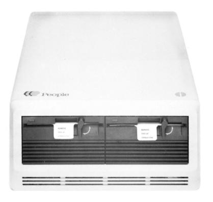
MAIN UNIT with inserted transport safety devices for read/write head
