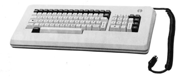
The keyboard contains 91 keys and is connected to the main unit by a coil cable.
