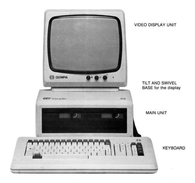
The separate, flat keyboard contains three key fields: an alphanumeric key field, a numeric key field, and a function key field. The alphanumeric keys correspond to regular typewriter keys for typing text in upper and lower case. A numeric key field facilitates entering numbers quickly. The definition of the individual
