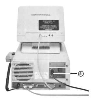
Plug 5 to connect the power supply
