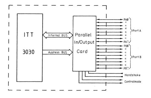
Fig.1: ITT 3030 with the Parallel Input/Output Interface
