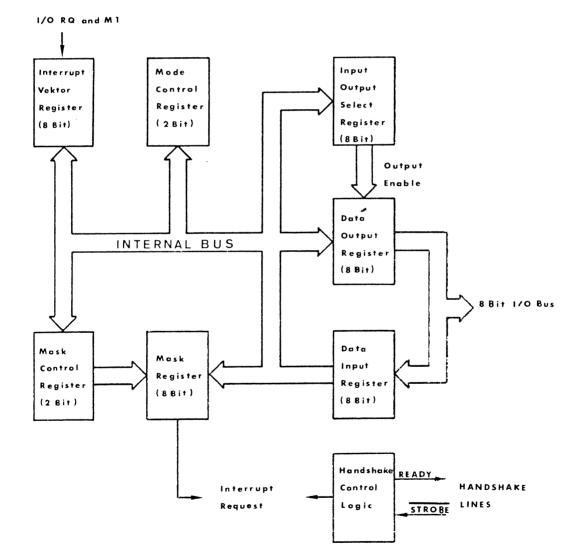
Fig.5: Detailled Block Diagram of an Input/Output Port
