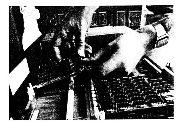
Fig.3: Installation of the PIO PCB - 6 - 7. Addressing
