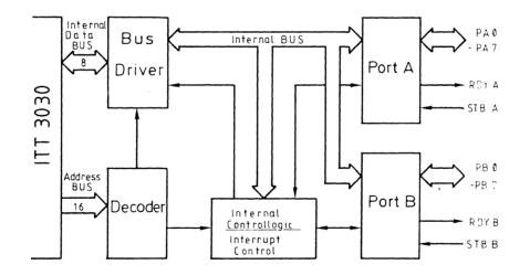
Fig.2: Block Diagram of the Parallel Input/Output Interface
