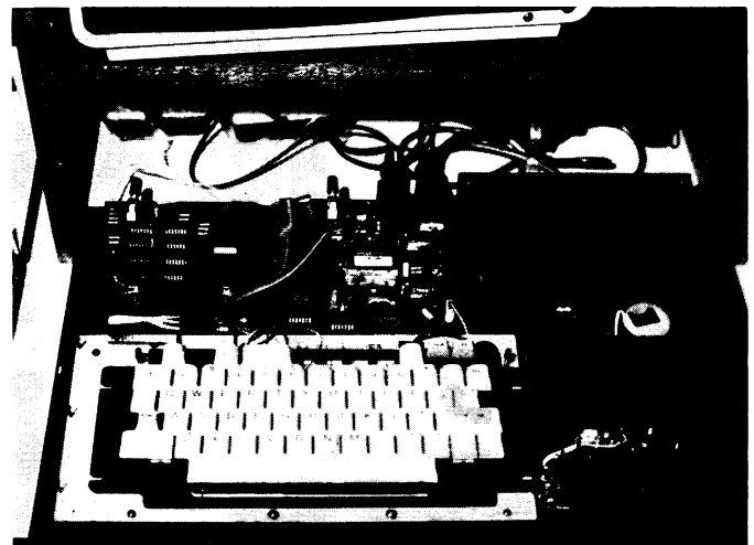
Into the interior, showing enclosed power supply and cassette recorder on the right, interface board with tv modulator at the center, the CPU board on the left. The Z80 is partly obscured by the ribbon cable from the keyboard.
