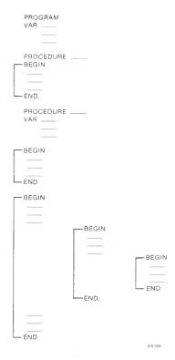
Figure 1-1. Block-structure in Pascal/MT+
