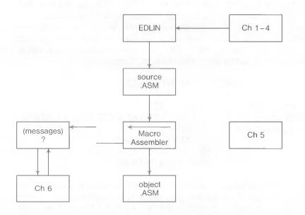
Figure 4. Overview of Macro Assembler Operation
